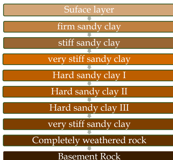
Figure 03-3 General soil layer description of the site.
